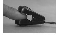
Figure 2. Infrared transmitter and received sensor pair clipped to the finger
