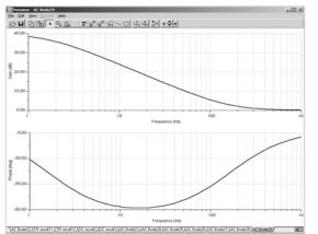
Figure 4. Frequency and phase responses of the amplifier and filter circuit (obtained by connecting a PC based oscilloscope to the circuit)
