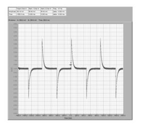
Figure 5. Output response of the amplifier and filter circuit (obtained by connecting a PC based oscilloscope to the circuit)
