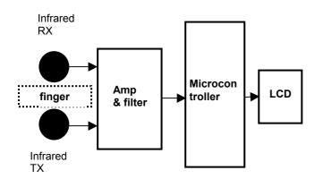
Figure 1. Block diagram of the measuring device
